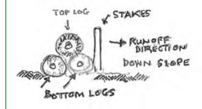
• If length is greater than 10', stagger joints so no 2 align.
